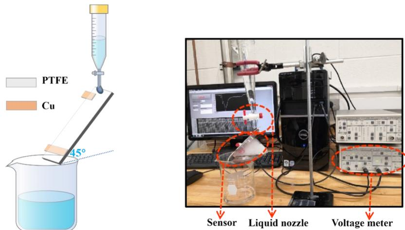
**Figure S1.** The schematic configuration and experimental setup of the TE-based liquid sensor.
