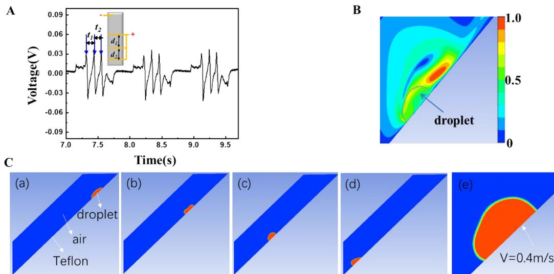
**Figure S4. The velocity result at the 45° inclined angle.** A. The voltage signals from multiple Cu electrodes. B. The velocity contour of the droplet and the air flow surrounding the droplet. C.(a) the expression of the CFD. (a-d) The dynamic features of the droplet at different time when it slides down the slope. (e)The close-up view of the droplet motion feature in (c).
