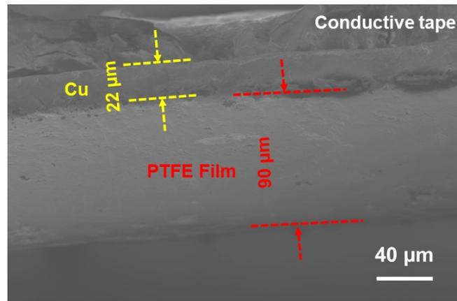
**Figure S2.** A cross-sectional SEM image of a TE-based liquid sensor.
