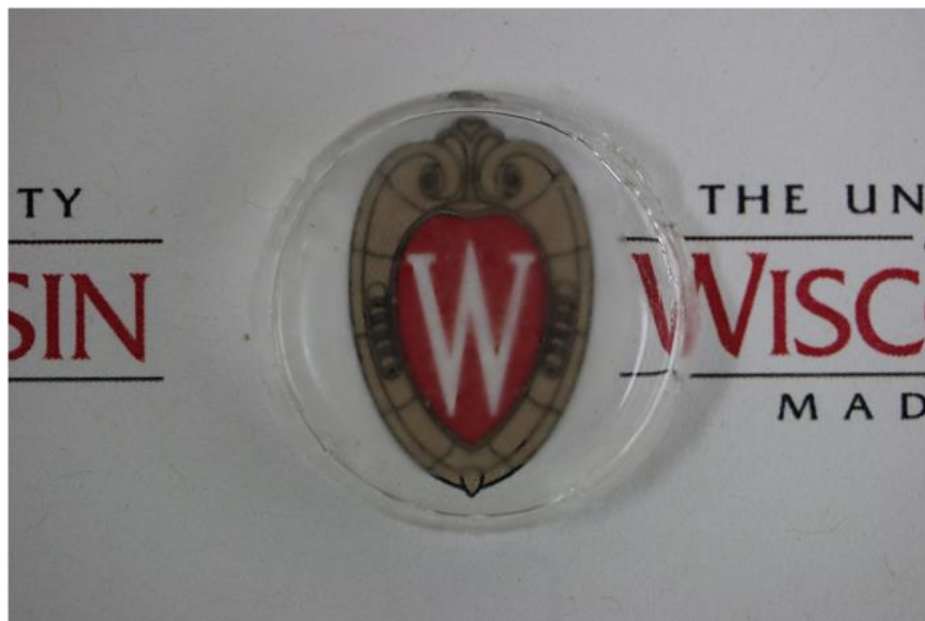
Figure S6. Disk-shaped PVDF-PDMS composite sample for compressive stress-strain test.
