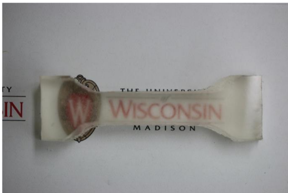
Figure S5. Dumbbell-shaped PVDF-PDMS composite sample for tensile stress-strain test.
